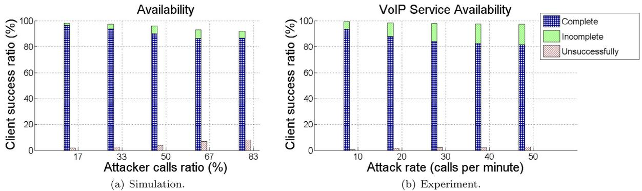
Fig. 17. Client success ratio: comparison between simulation and experimental results for lognormal call duration when using SeVen with a tournament dropping strategy.
