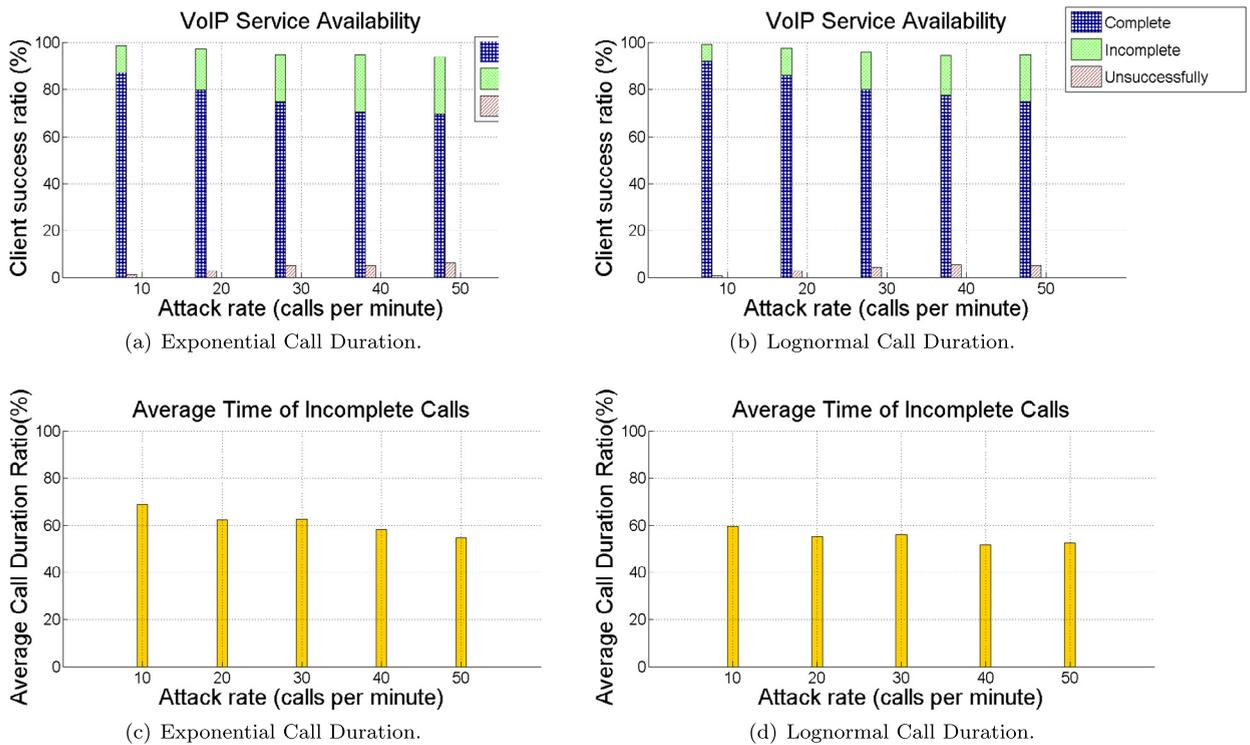
Fig. 12. Client success ratio and average time of incomplete calls: experimental results when using SeVen with a roulette dropping strategy.
