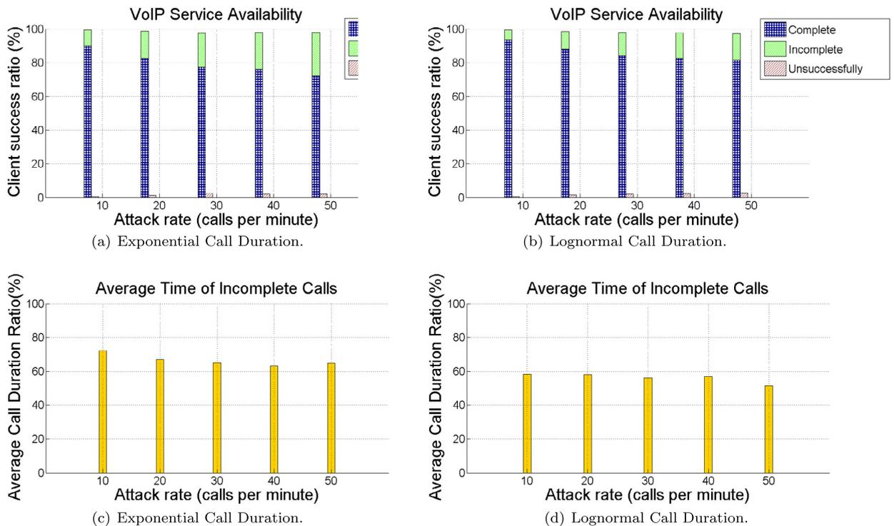
Fig. 14. Client success ratio and average time of incomplete calls: experimental results when using SeVen with a 100-tournament dropping strategy.
