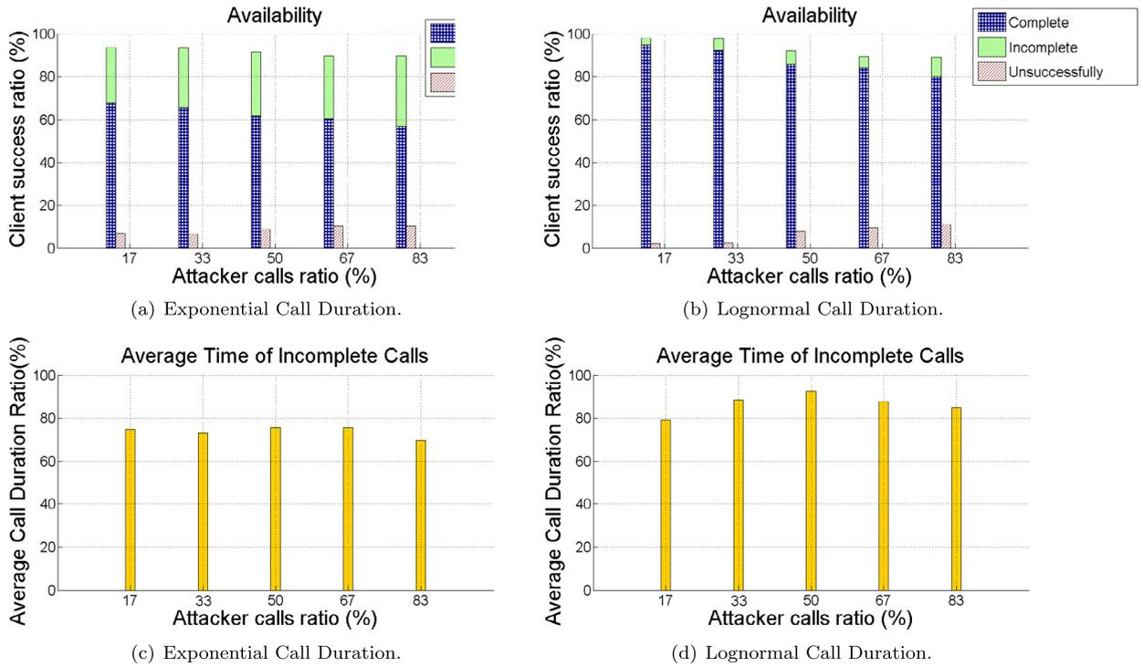
Fig. 6. Client success ratio and average time of incomplete calls: simulation results when a roulette dropping strategy.
