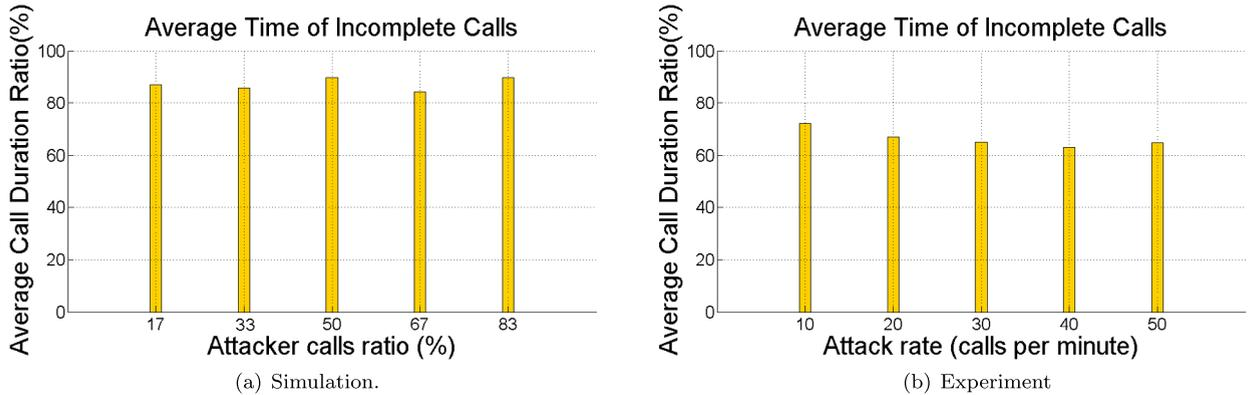
**Fig. 18.** Average time of incomplete calls: comparison between simulation and experimental results when using SeVen with the  $\frac{k}{2}$ -tournament dropping strategy.
