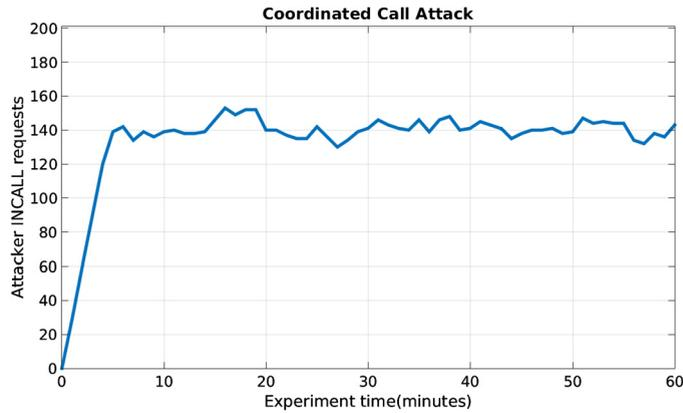
Fig. 15. Attacker call occupancy in buffer: experimental results when using SeVen with a 100-tournament dropping strategy.
