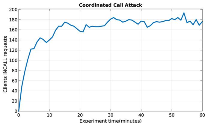
It shows that the server is indeed well dimensioned for this rate of (legitimate) calls. Clients occupy in average approximately 85% of Asterisk's capacity thus not overloading the server, but still being heavily used.
