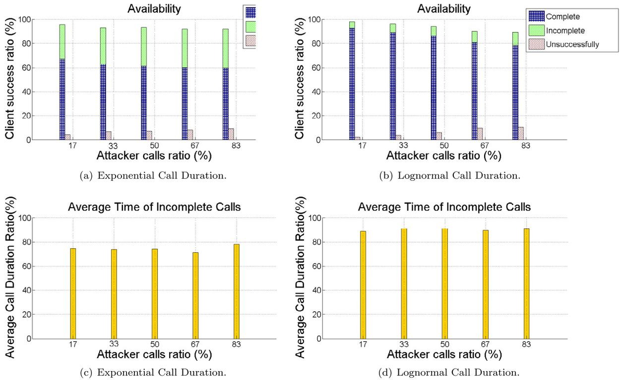
Fig. 5. Client success ratio and average time of incomplete calls: simulation results when a uniform dropping strategy.
