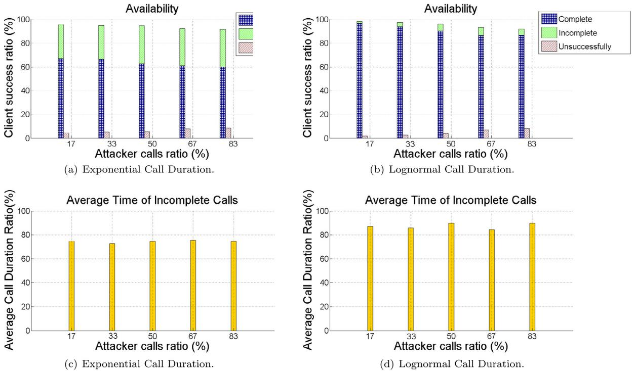
Fig. 7. Client success ratio and average time of incomplete calls: simulation results when using a tournament strategy.
