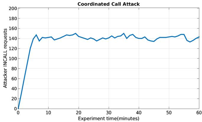
Fig. 13. Attacker call occupancy in buffer: experimental results when using SeVen with a roulette dropping strategy.
