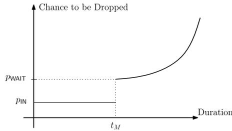
**Fig. 2.** Graph (not in scale) illustrating the behavior of SeVen according to the status of a call and its duration.  $p_{\text{WAIT}}$  is the probability of dropping a WAITING call, while  $p_{\text{IN}}$  the probability of dropping a INCALL call.
