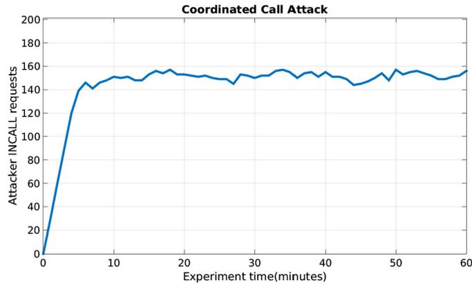
Fig. 11. Attacker call occupancy in buffer: experimental results when using SeVen with a uniform dropping strategy.
